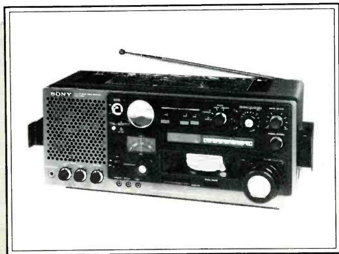
The Sony ICF-6800W is fully portable with its own whip antenna and offers a number of base station features.
